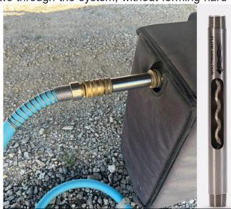
A departure from salt regeneration water systems is the NaturalSof NS-RV Water Conditioner, a 3-inch inline device that uses a catalytic process through a metal core that prevents calcium from bonding. In other words, the calcium remains suspended and flows out with the water. It's not cheap but eliminates the use of salt and backflushing — and also requires no power.
